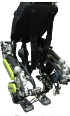
The lower-body strength-augmenting exoskeleton "XO"
